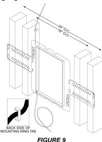
9), such as the M&S Systems MS16X. for attachment to the speakers after the dry wall has been installed. Leave at least 18 inches additional cable for the connection during final speaker installation. Run the other end of the speaker cable to the audio source.
